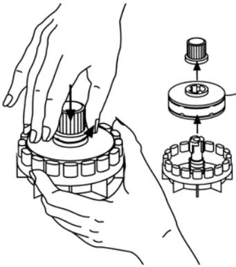
**Note:** If the tap button cannot be pressed down, turn the cord cartridge to the right or left until it stops. Then proceed as described above.
