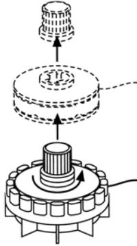
5. Press the cord cartridge down against the spring and fix it in this position by a short turn to the left or right.
