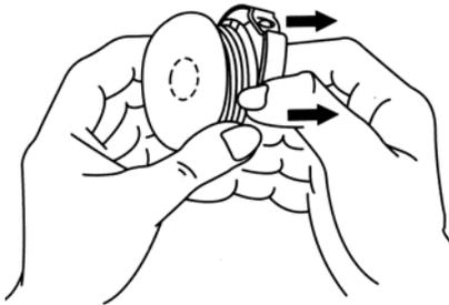
4. The reel of trimmer cord is now open. Reel off approximately 10 cm (4 inches) of trimmer cord and clamp it in the notch on the spool.
